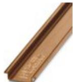
DIN rail, unperforated, Standard profile, width: 35 mm, height: 7.5 mm, acc. to EN 60715, material: Copper, uncoated, length: 2000 mm, color: copper-colored
