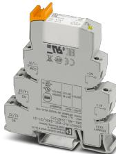
PLC-INTERFACE, consisting of PLC-BSC.../21 basic terminal block with screw connection and plug-in miniature relay with multi-layer gold contact, for mounting on DIN rail NS 35/7,5, 2 changeover contacts, input voltage 24 V DC
